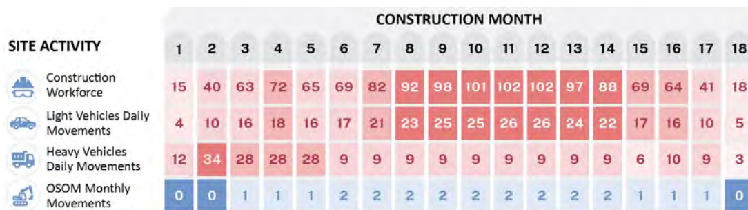
Figure 3.4 Construction Workforce and Traffic Movements
