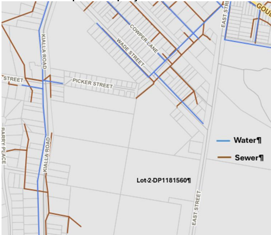
Figure 3: Location of Council's Water and Sewer Reticulation System in Respect to Development Property
